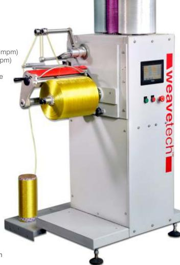
9000 x Feed Wgt in gms Denier x Yarn Speed in mtrs/min
